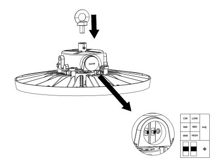
As shown in the figure, unscrew the plug of driver housing, toggle the dip switch to adjust the required CCT/Power and screw on the plug.
